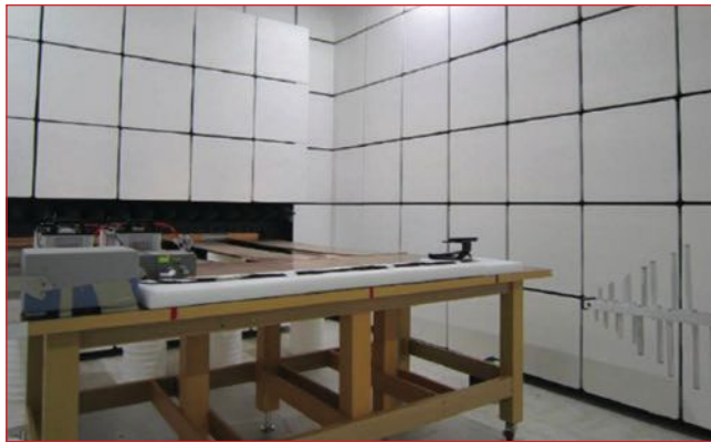
▲ Fig. 3 Radiation measurement setup showing log-periodic antenna.
