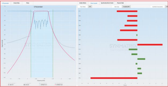
▲ Fig. 3 AI-optimized results for edge-coupled bandpass filter structure.
