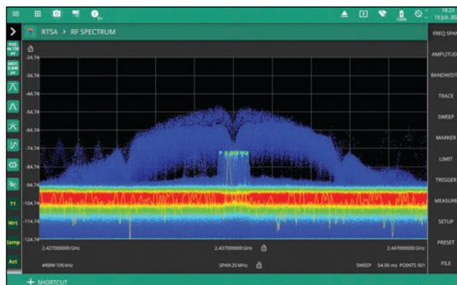
▲ Fig. 3 Pulsed signal hidden in an ISM-band Wi-Fi carrier.
